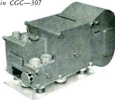
The Century Model 409 Oscillograph has been designed for recording data where space and weight requirements are limited. The Oscillograph has been tested to record faithfully while subjected to accelerations up to 20 G's.
