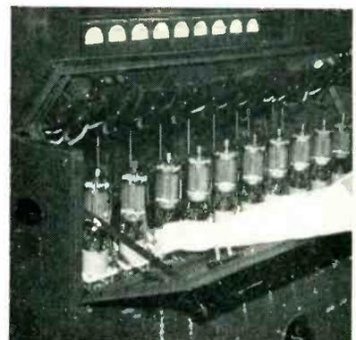
Safety-first console developed for testing ten large tubes at a time without risk of electrical shock to the operator
