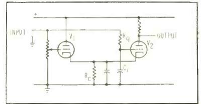
FIG. 3—Pulse-width discriminator circuit
