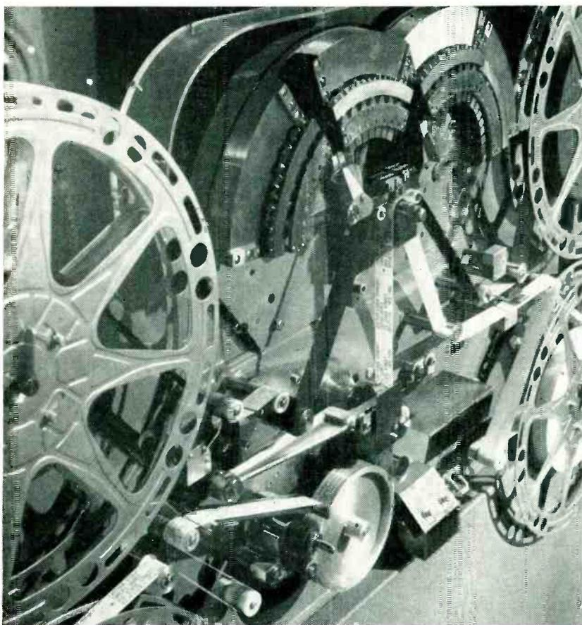
Printing styli strike impact blows on paper through carbon; each of four printing heads prints one line of address
