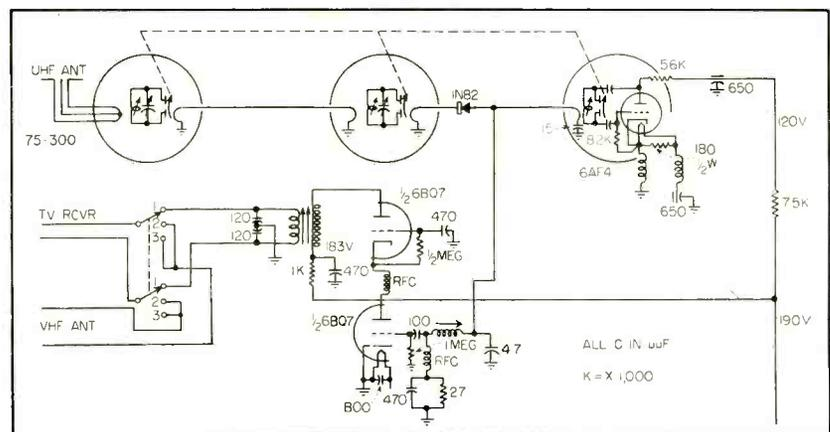
FIG. 4—Converter circuit includes cascade i-f stage
