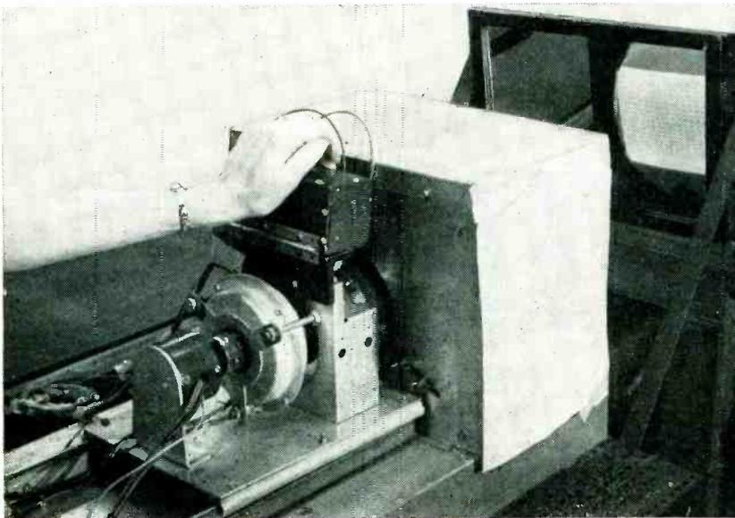
Crosley-developed test set for deflection yokes, with slant-line pattern for good yoke showing in mirror at upper right. Operator must press down cover of switch against spring action as shown in order to apply power for test
