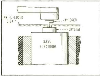
FIG. 5—Mounting and contacts for crystal triode
