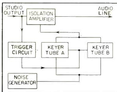
FIG. 1—Block diagram showing portion of generator used to furnish reverberation to gunshot by inserting a decaying random-noise signal after the actual shot signal
