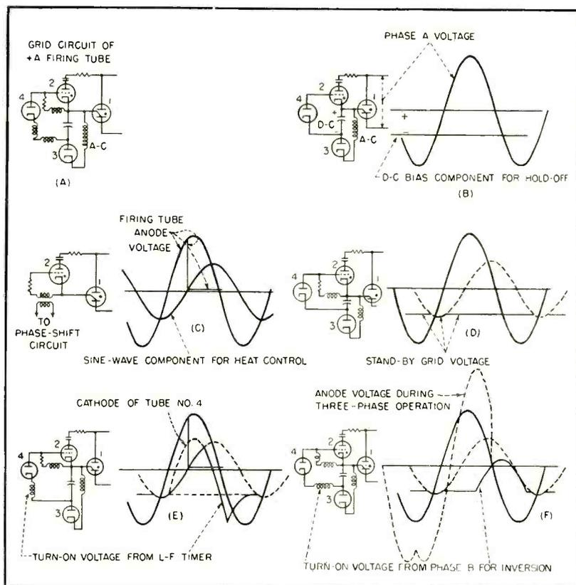
FIG. 7—Analysis of firing-tube grid circuit for turn-on, heat control and inversion
