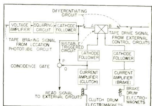
FIG. 3—Electronic control system for tape feed
