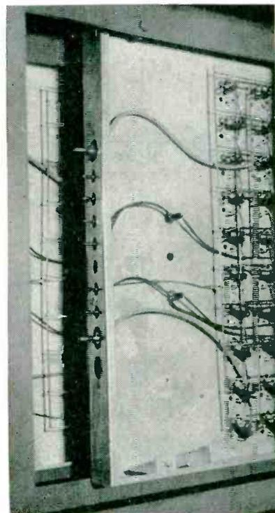
Rear view of slide-out aging drawer, showing jacks that make connections to mating jacks at rear of rack. Supporting rollers are at top of drawer and locking latch is at bottom
