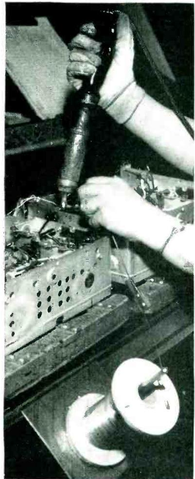
Use of inexpensive angle brackets on pallets to position auto radios, and simple support for solder reel. The solder holder can be slid along the bench readily, and may be lifted off when no longer needed.
