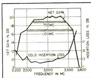
**FIG. 5—Net gain and cold-insertion loss curves vary owing to imperfect match between helix and coaxial input and output lines**
