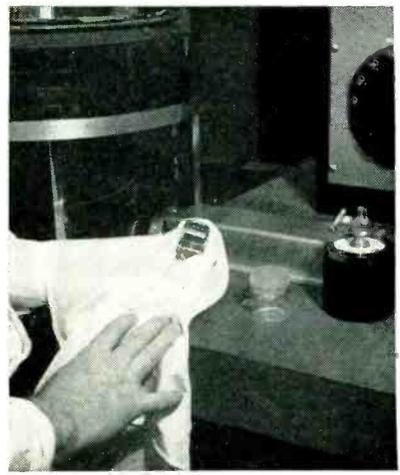
Method of handling baked-out parts with a lint-free cloth. Glass container is used for storage before baking, and container at right is used after bake out
