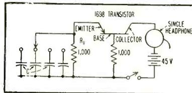
FIG. 1—Circuit of R-C oscillator for toy transistor organ
