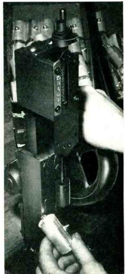
Upside-down scale operated by rack and gear measures downward testing pressure being applied to plunger in pencil triode cavity. New printed numbers have been placed on scale so operator does not have to read upside-down values
