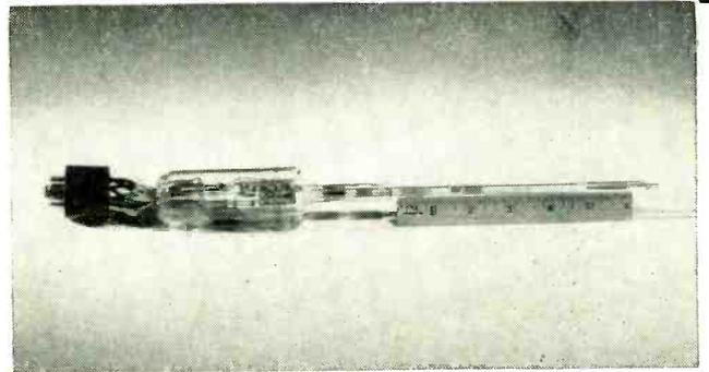
FIG. 2—Short tube uses folded-back antenna, bypass sleeve for input and collector for output coupling
