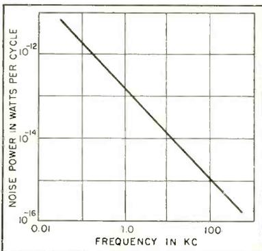
FIG. 1—Inverse relationship of transistor noise power per unit bandwidth and frequency
