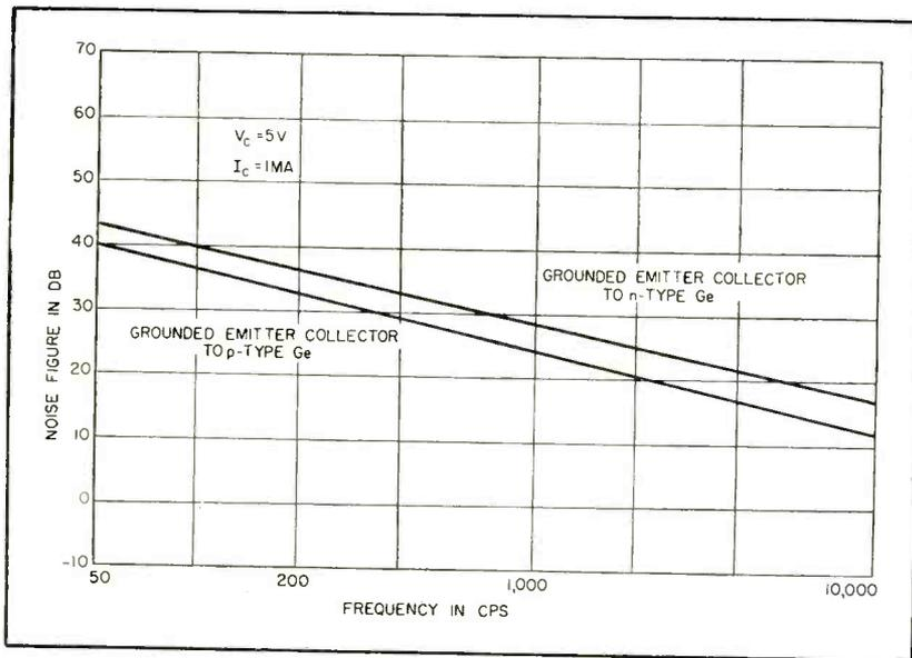
FIG. 3—Variation of noise figure with frequency for two different types of junction transistors
