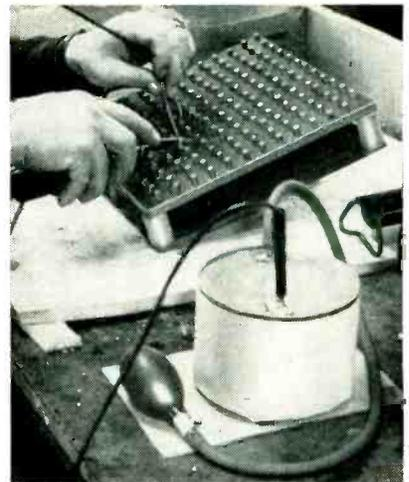
Improved water cooling system using one-pound coffee can in foreground as reservoir. Water hose goes to resistance soldering tool in operator's right hand. Jig for supporting the plugs during soldering is made from heat-resisting material and has drilled holes to take 168 plugs at a time. Surplus water runs down angle-mounted jig onto rubber-sponge mat on bench
