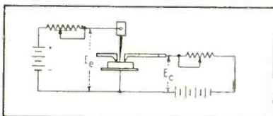
FIG. 6—Circuit of the disk-contact crystal triode
