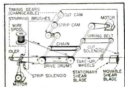
Operating principle of high-speed continuous wire stripping and cutting machine, in which gear-driven cams control operation of the stripping and cutting solenoids
