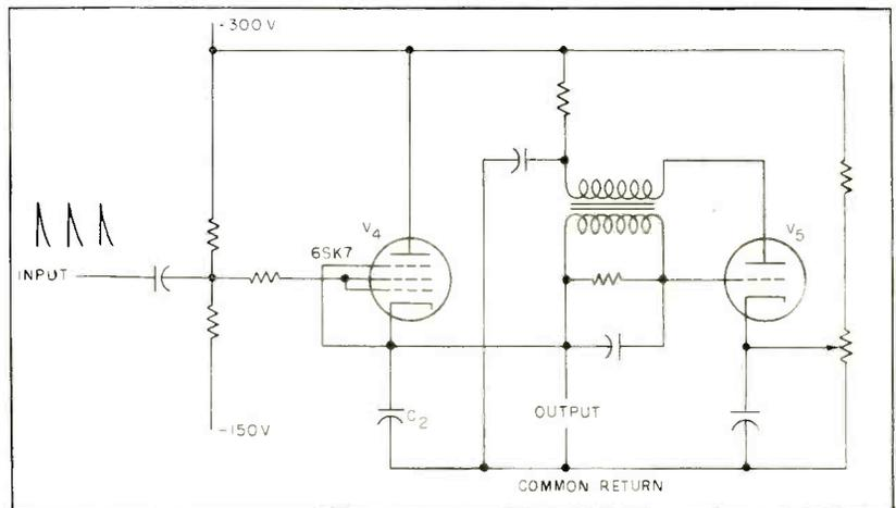
FIG. 6—Staircase generator steps bias current automatically to display family of transistor characteristics
