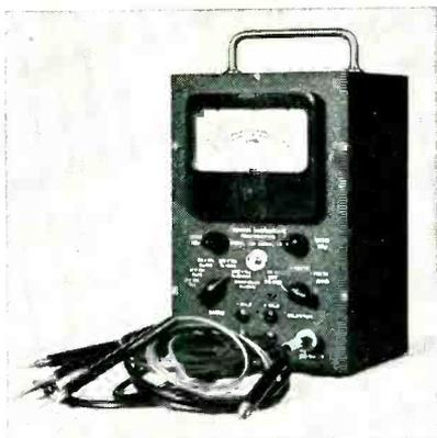
Model 601 Vacuum Tube Volt-Ohm-Milliammeter
