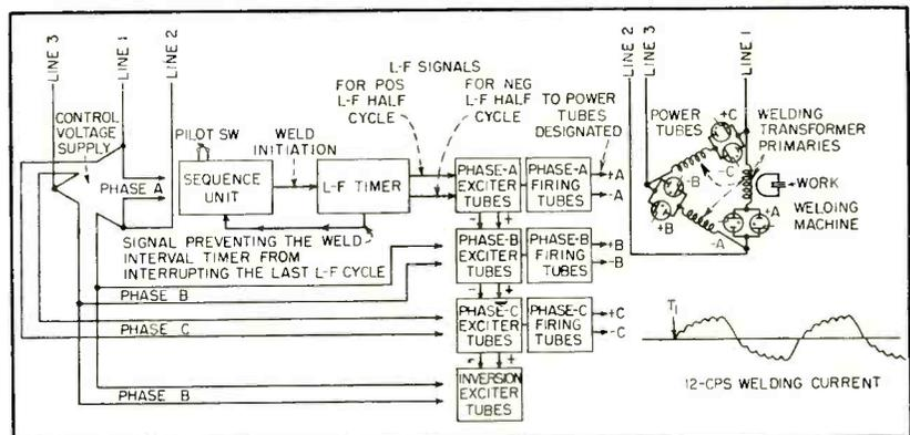
FIG. 5—Control and power circuit sections and basic mode of operation
