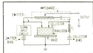
FIG. 9—Transistor amplifier uses impedance between emitter and collector
