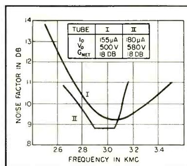
**FIG. 6—Noise figures of two tubes as function of frequency**
