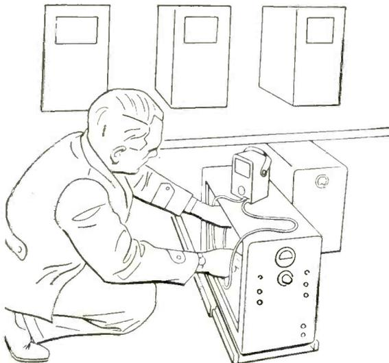
Picture distribution amplifier unit as well as synchronizing generator and power supply units are mounted on Grant Industrial Slides. Units are normally retracted but roll out for servicing.
