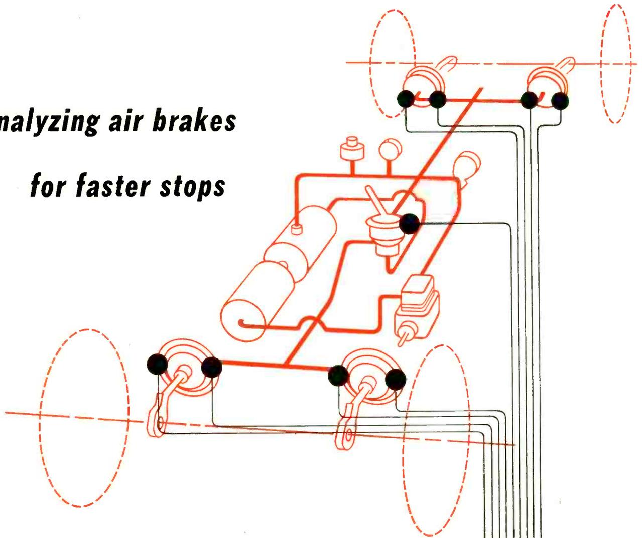
How LONG does it take pressure to build up to required levels at the brake chambers after the driver applies the brake pedal? To answer this all-important question of "air-transmission" time, Bendix-Westinghouse Automotive Air Brake Company assembles on a test stand a complete counterpart of the brake system which is to be installed in a truck, truck-tractor, or bus. All components and air lines are the same as those to be used on the vehicle.
