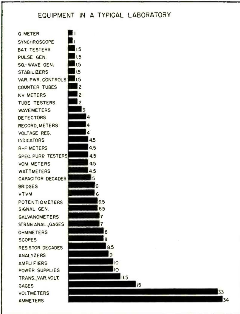
Survey by ELECTRONICS of 459 laboratories in 10 different classifications shows they contain 116,395 instruments. Identity of 36 types is shown above. Remaining types average less than one and include field-strength meters, spectrometers, sweep calibrators, colorimeters and radiation meters
