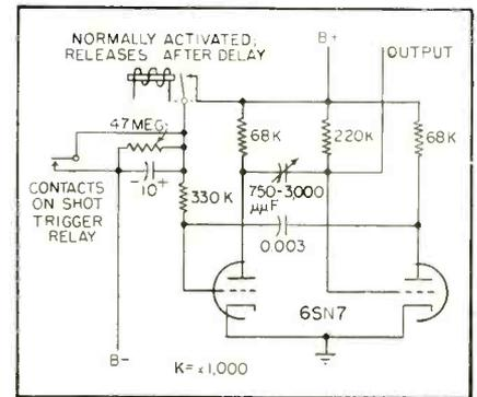
FIG. 5—Ricochet delay relay circuit and associated double-triode oscillator
