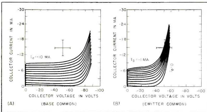
FIG. 7—Transistor-curve tracer implements study of collector breakdown voltage under varying bias conditions
