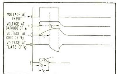
FIG. 4—Waveforms show operation of discriminator
