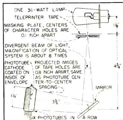
FIG. 6—Optical system of reader
