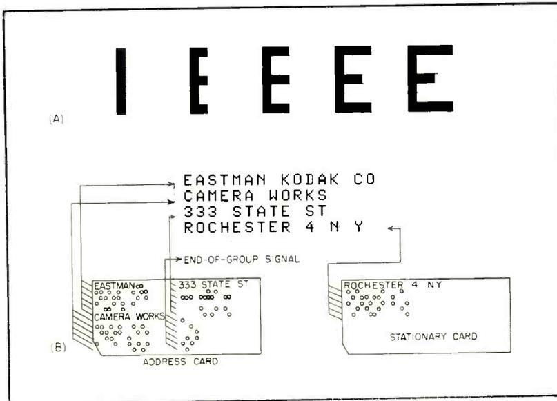
FIG. 1—Letter E is built up on 35-dot matrix (A) in five blows by printing styli. Punch cards (B) are quartered to give four-line address of 24 characters per line. Alphabetical and numerical characters are expressed in six-unit code
