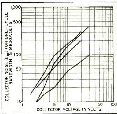
FIG. 5—Open-circuit collector noise voltage for four different point-contact transistors
