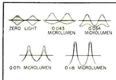
FIG. 2—Envelope patterns at the anode of the multiplier phototube
