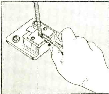
**1** Truarc applicator is pushed forward and grips a single E-ring.
