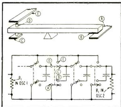
FIG. 3—More elaborate keyboard permits playing of two notes simultaneously with a single set of frequency-determining capacitors. Circled letters on key refer to points on circuit below
