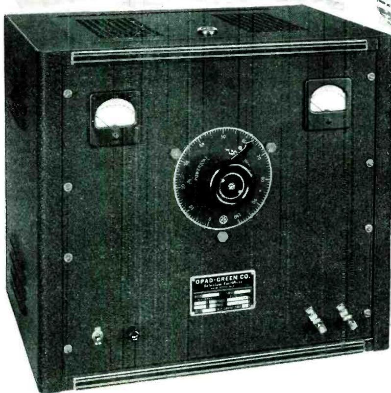
The OPAD-GREEN General Purpose Power Supplies are designed to furnish an adjustable source of unfiltered direct current from single phase 50 or 60 cycle A.C. power lines. A unique feature is their stepless control of the D.C. output voltage which permits them to serve as power sources for a wide variety of electrical equipment and electro-chemical processes. *For additional information write for Bulletin No. 147*
