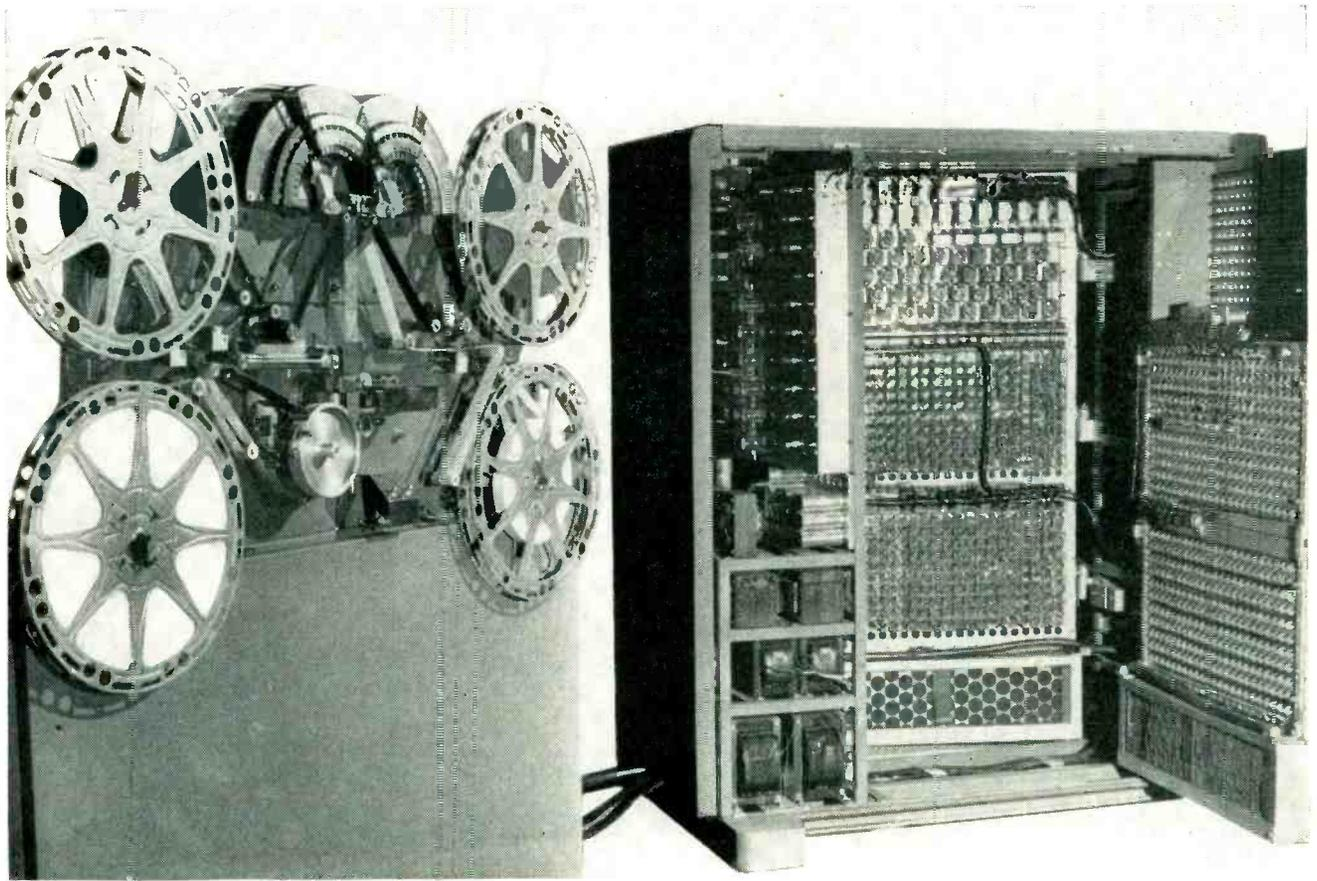
Multiple-stylus printer has punch-card feed and photoelectric card reader located behind printing unit (left). Electronic unit converts punch-card data to impulses that drive printing styli
