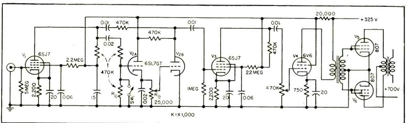
FIG. 3—Typical 50-watt modulator built around compressor circuit. Resistor  $R_2$  (Fig. 1) can be omitted for speech work
