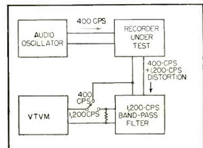
FIG. 1—Block diagram of distortion measuring system
