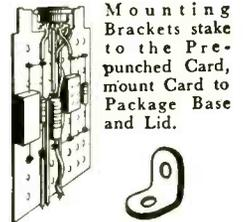
Mounting Brackets stake to the Pre-punched Card, mount Card to Package Base and Lid.
