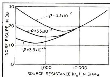
FIG. 10—Variation of noise figure with source resistance for different values of  $E_{ne}/E_{nc}$
