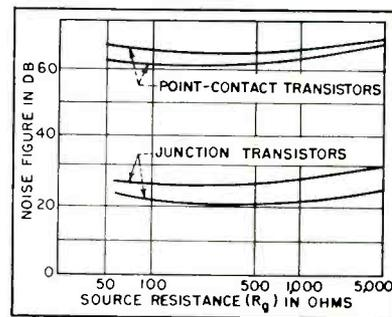
FIG. 11—Comparison of noise figure in point-contact and junction transistors
