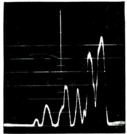
False-echo return due to scattering at air-water interface. Lock-out bars all but shortest-path echo
