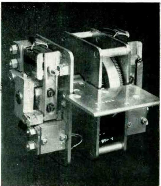
Tape feed assembly; brake drum and braking solenoids are at left, and clutch drive system is at right
