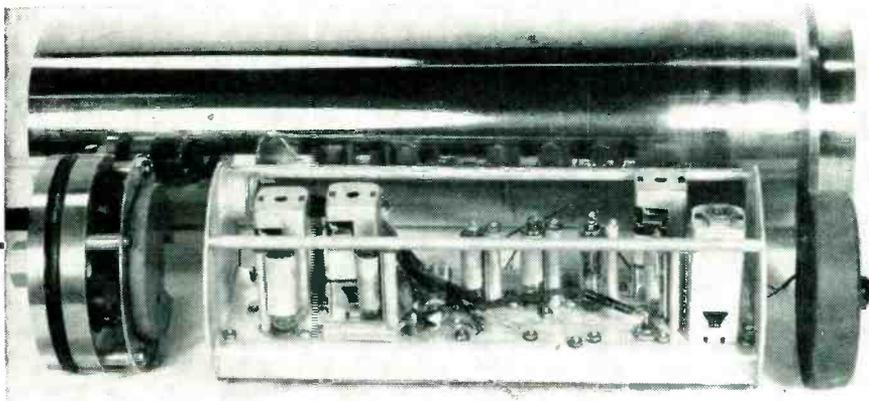
Depth recorder chassis is mounted in watertight cylinder with acoustic transducer forming top of can
