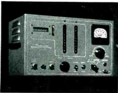
The DS-606 is a versatile laboratory scaler easily adaptable to GM and scintillation counting and frequency checks. Pulse height discriminator from 0 to 100 volts; position or negative pulses. It has a high voltage power supply which is variable in one step from 0 to 2.5 KV. The power can supply either the GM input or can be used as a power source for accessory equipment.
