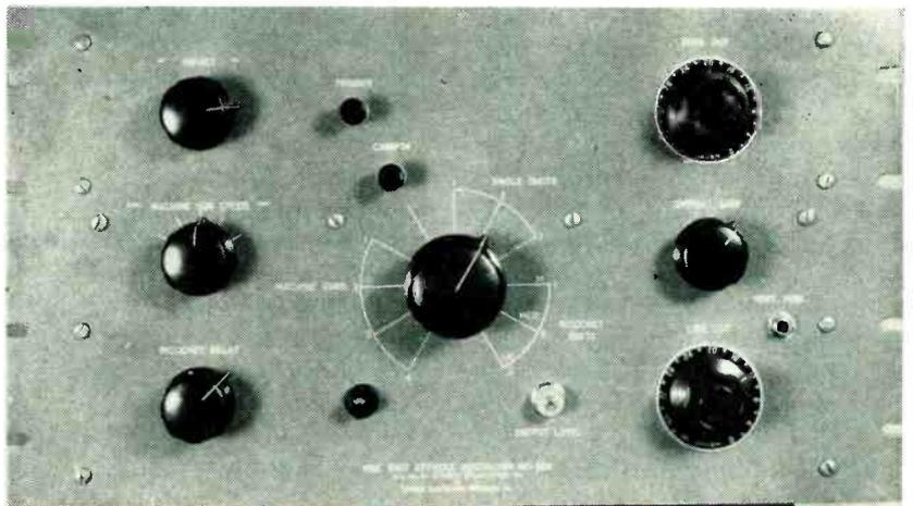
Front-panel controls of generator permit quick setting to give variety of shot effects
