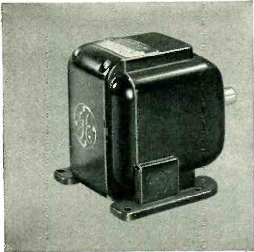
**PLUGGING CONTROLS**—New device for brakeless stopping of motors features Carboloy magnets. Eddy-current disk rotates in magnetic assembly, creates torque. As motor's speed nears zero with power reversed, torque interrupts circuit, cuts stopping time from 20 seconds to 1 second.
