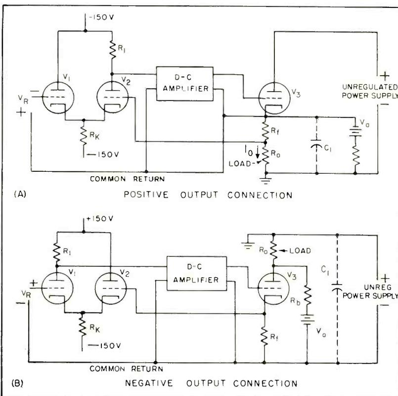
FIG. 5—Current regulator supplies either positive or negative constant-current bias to transistor's unswept terminal
