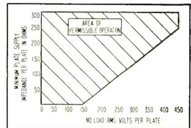
FIG. 3—Operation for hot-switching current of 1.8 amp
