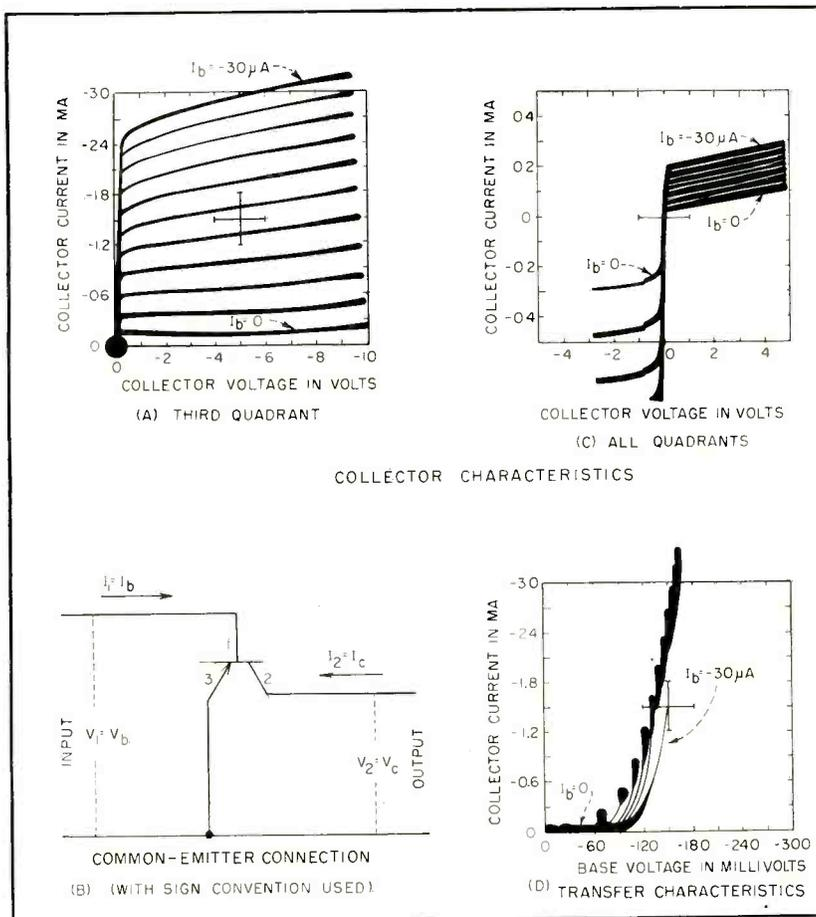
FIG. 2—Collector and transfer characteristics for junction transistor with common-emitter connection (B). Collector curves are shown for negative current and voltage (A) and for all quadrants of volt-ampere coordinate system
