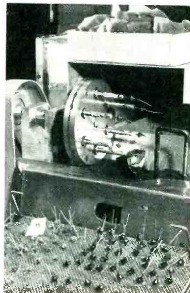
Machine with container of hot wax raised to dunking position. U-shaped metal bar comes up with pot, to serve as guard, because the wax is hot enough to burn fingers
