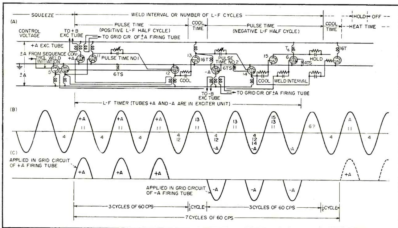
FIG. 9—Low-frequency timing circuit
