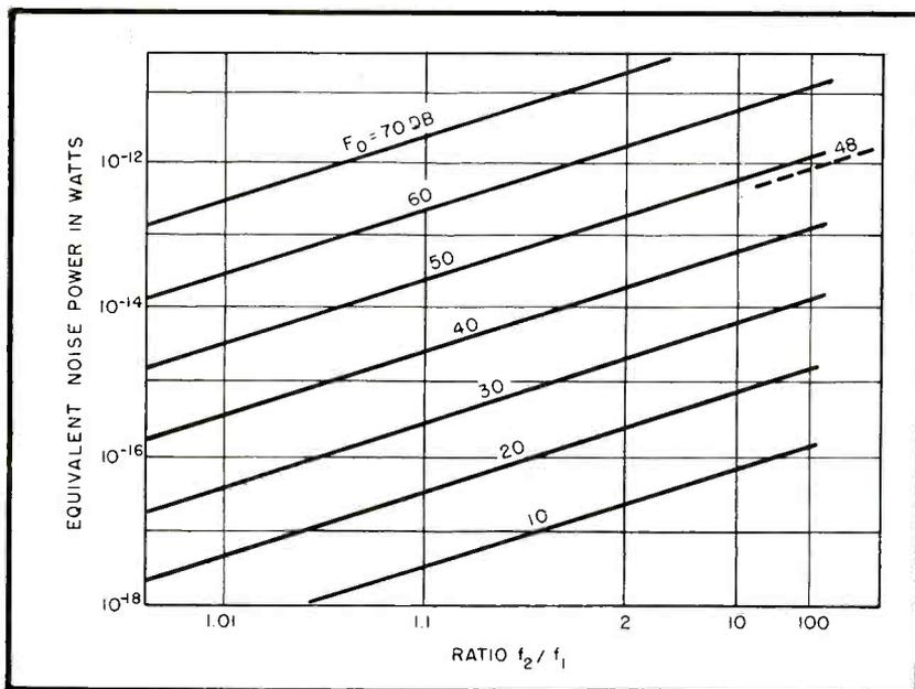
FIG. 9—Available equivalent noise power
