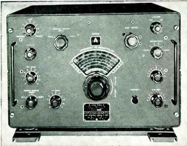
Radio Receiving Set, R-366/TRR5, a 14-tube superheterodyne with a frequency range of 540-30,000 kilocycles covered in five bands. Courtesy Espey Mfg. Co., New York
