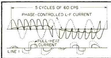
FIG. 2—Phase-controlled power tubes determine the effective value of the single-phase low-frequency voltage
