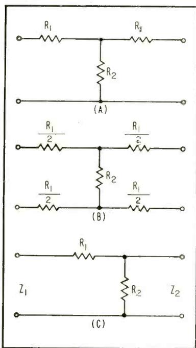
FIG. 1—Values of resistors for T-type (A), H-type (B) and low-loss L-type (C) pad attenuators can be determined from Table I
