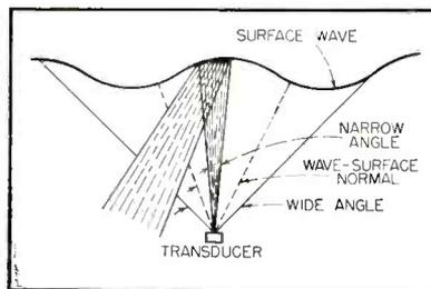
FIG. 6—Transducer sacrifices directivity to reduce loss of echo due to torpedo roll and pitch
