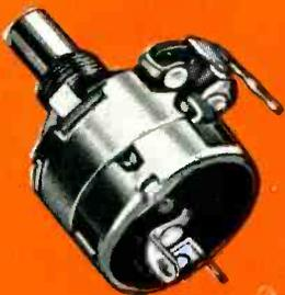
TYPE GC-45, 15/16" diameter variable composition resistor. Wattage ratings: 1/2 watt for resistances through 10,000 ohms, 1/3 watt for resistances over 10,000 ohms through 100,000 ohms, 1/4 watt with 500 volts maximum across end terminals for resistances over 100,000 ohms. Available with or without illustrated attached switch and in concentric shaft tandem construction C2-45 as shown above.
