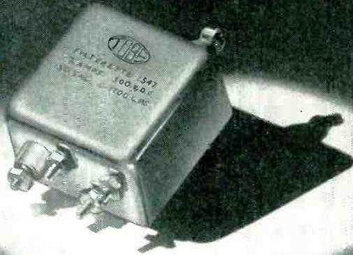
In a space only  $2\frac{1}{2}'' \times 2'' \times 1\frac{3}{16}''$ , you can get better than 85 db attenuation throughout most of the useful range up to 1000 megacycles by using any one of the #1547 series of Tube interference filters. With their extremely low series resistance, these effective filters have negligible voltage drop and only slight temperature rise. Hermetically sealed, Series 1547 filters meet military specifications for use from 55C to  $-105C$ .
