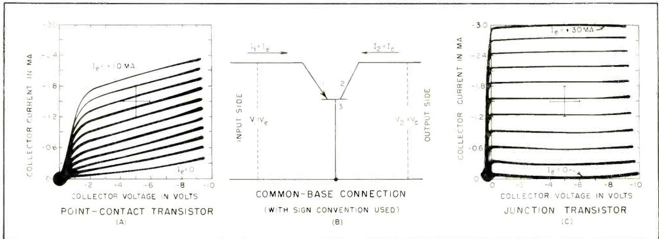
FIG. 1—Transistor output characteristics. Schematic (B) shows common-base connection used in deriving curves for point-contact transistor (A) and junction type (C)
