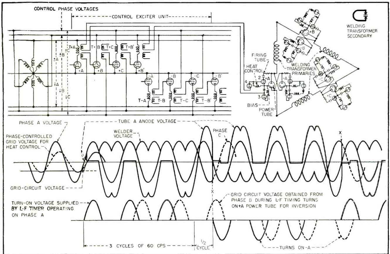
FIG. 6—Details of exciter unit circuit and power circuit, including firing tubes
