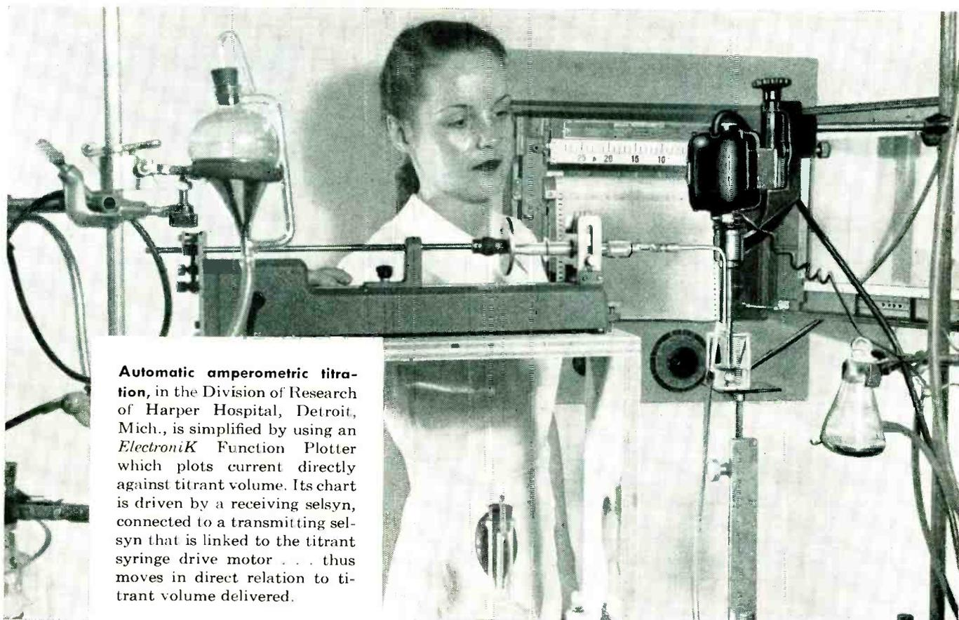
**Automatic amperometric titration**, in the Division of Research of Harper Hospital, Detroit, Mich., is simplified by using an *ElectroniK* Function Plotter which plots current directly against titrant volume. Its chart is driven by a receiving selsyn, connected to a transmitting selsyn that is linked to the titrant syringe drive motor . . . thus moves in direct relation to titrant volume delivered.
