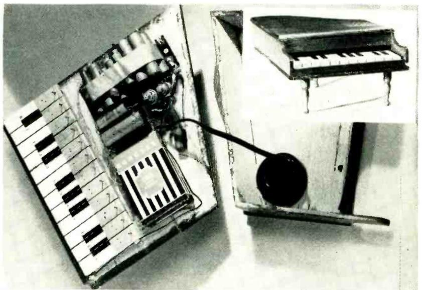
Transistor organ uses a toy piano case and keyboard (see inset upper right) for all components and battery shown in principal photograph. Single headphone is mounted against top (at right)
