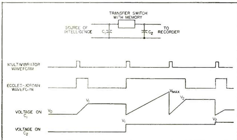
FIG. 5—Boxcar demodulator holds Eccles-Jordan output during repetition intervals in which echo is lost
