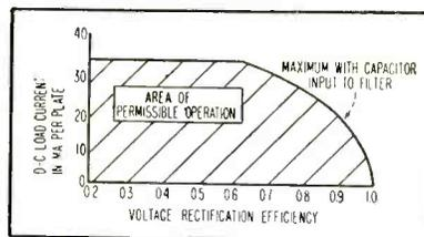
FIG. 2—Load current vs efficiency for 6X4 for 210 ma peak steady-state current
