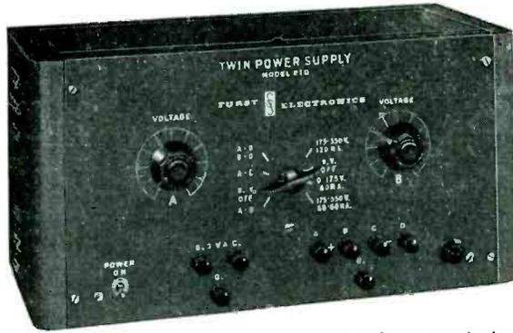
Two independent sources of continuously variable D.C. are combined in this one convenient unit. Its double utility makes it a most useful instrument for laboratory and test station work. Three power ranges are instantly selected with a rotary switch:
