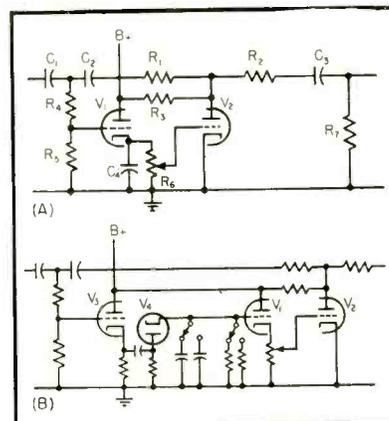
FIG. 2—More elaborate circuits prohibit distortion by input loading and extend frequency response
