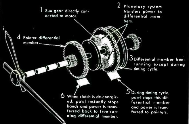
In this unique clutch mechanism, the motor is permanently connected to the sun gear of a differential gear system. A solenoid pawl moves between the two differential members so that only one is free to rotate at one time. Starts and stops are thus effected by positive engagement of pawl with gear. There can be none of the slippage or overrun associated with friction clutches; nor can characteristics change with age.
