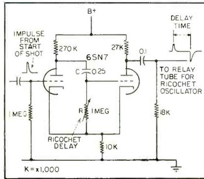
FIG. 4—Delay multivibrator circuit in simplified form, with pulse waveform
