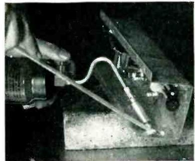
Tinning an aluminum radio chassis by heating with a gas torch and rubbing the heated area with a rod of the new alloy
