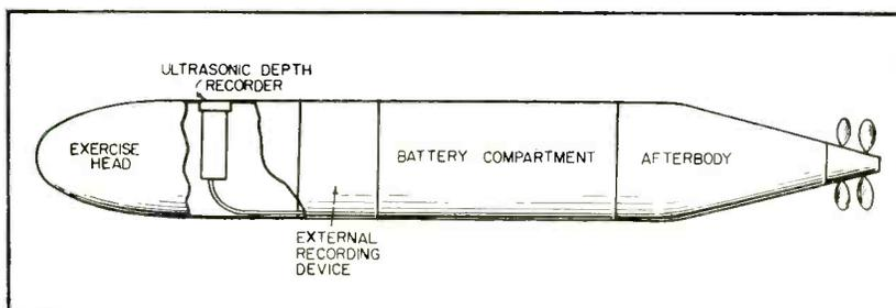
FIG. 1—Test torpedo fitted with exercise head. Cut-away shows depth recorder in place. Strip-chart recorder is forward of battery compartment
