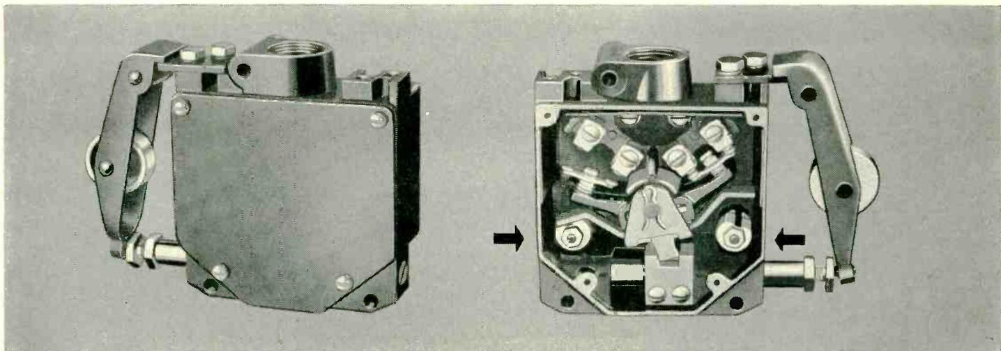
**LIMIT SWITCHES**—Even under severe service, this double-break switch will stand up well. Its 2 independent circuits are alternately held open and closed solely by small Carboloy permanent magnets. The magnets assure positive
