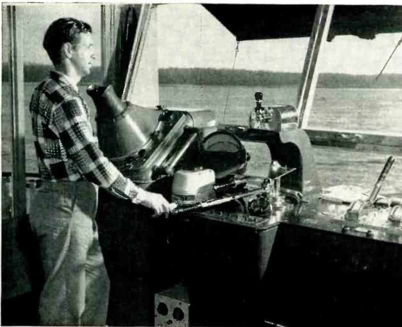
Modern Mark Twain can either steer or automatically hold a course with this new electronic pilot. Big-boat skippers can use it instead of shouting to the helmsman from the radar screen
