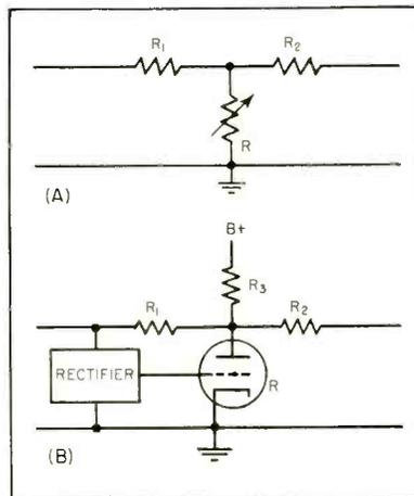
FIG. 1—Replacing it with signal-biased vacuum tube provides signal compression
