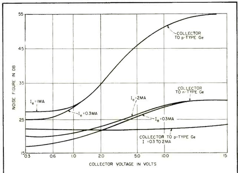
FIG. 7—Transistor noise versus operating point
