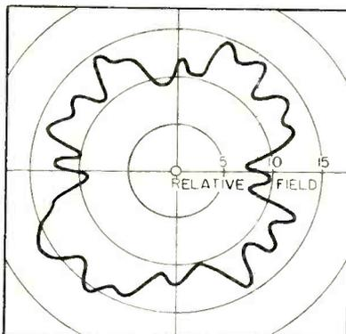
Measured pattern for 90-degree skewed antenna
