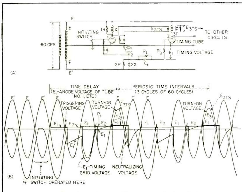
FIG. 8—Basic timing circuit used in low-frequency timing section
