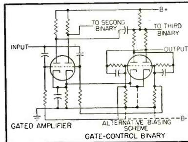
FIG. 2—Gated amplifier with paralleled grids is switched by gate-control binary
