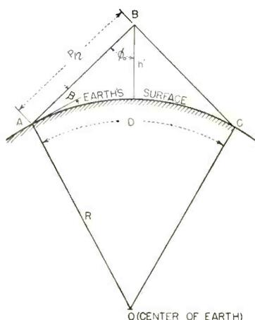
FIG. 1—Diagram shows geometry of sky-wave propagation
