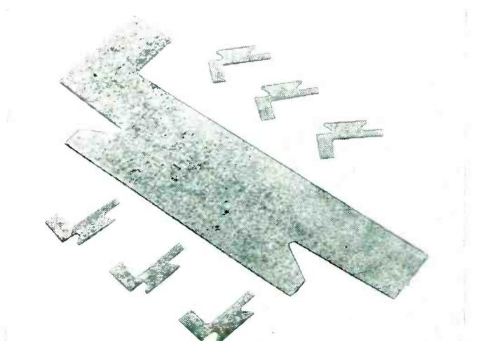
**4. Need a class H segment plate that's easy to work with?** ISOMICA\* Segment Plate — made of built-up continuous mica sheet — shows no tendency to split or flake. Small segments of heavy thickness may be punched, and larger segments can be accurately sawed, milled, punched, etc.
