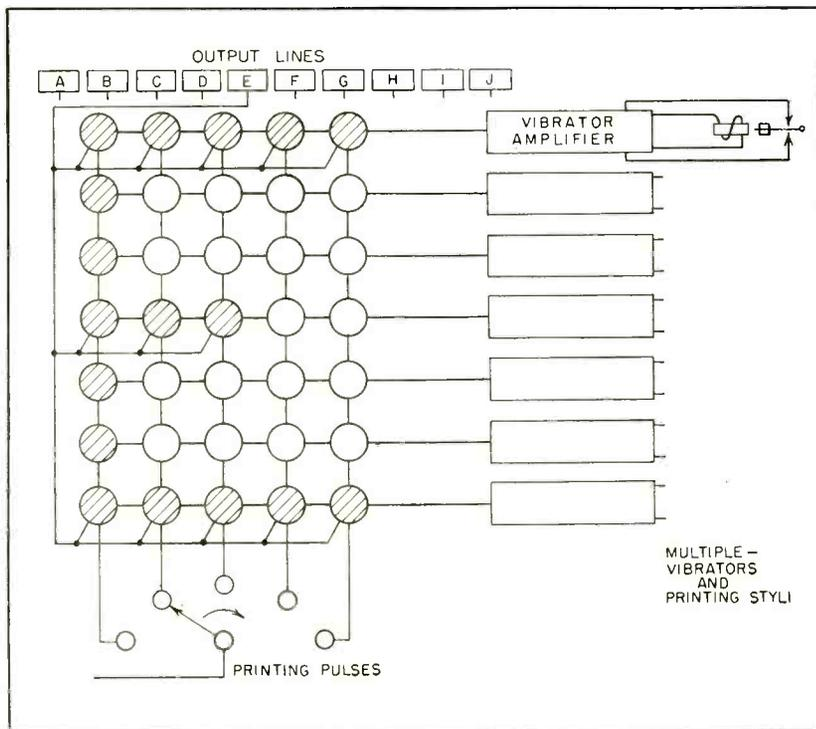
FIG. 2—Output lines from decoding matrix select pattern of switch combinations corresponding to desired character. Switch matrix columns are read out by five of the seven printer timing pulses
