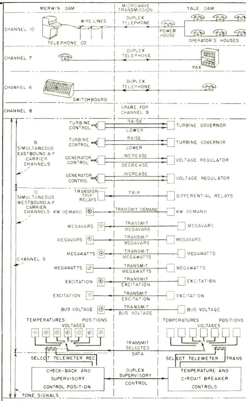
FIG. 1—Channel utilization in microwave control systems between Merwin and Yale dams shows functions possible with five existing subcarrier channels. Seven additional channels, not yet installed, can be made available
