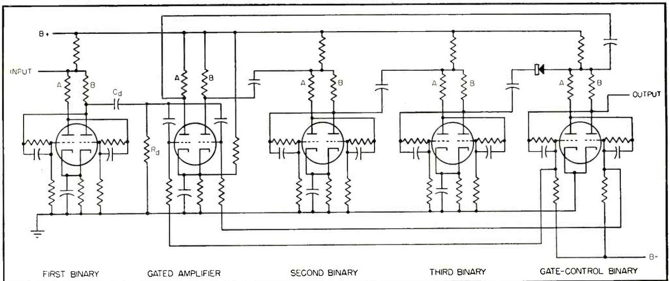
FIG. 3—Counting operation may be traced from circuit schematic. Eighth pulse flips third binary, which, in turn, flips gate-control binary. Gated amplifier feeds tenth pulse to gate-control binary resetting decade and producing output pulse
