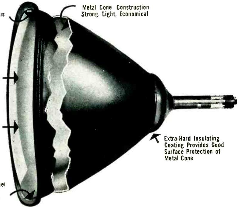
Extra-Hard Insulating Coating Provides Good Surface Protection of Metal Cone
