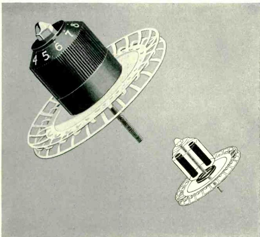
**TENSION BRAKES**—Three tiny Carboloy permanent magnets are used in this new magnetic brake that controls the winding of yarn and fine fibres. The magnets (shown in cutaway) provide even tension through magnetic drag, cut down on abrasion, slippage, static electricity—give wider tension and speed ranges. Carboloy permanent magnets never need maintenance, never fail.
