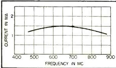
FIG. 3—Crystal injection current is nearly constant over the frequency range
