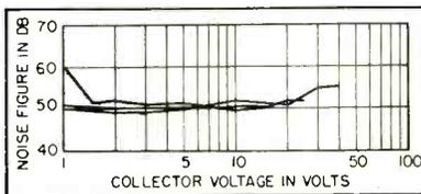
FIG. 6—Variation of noise figure with collector voltage for three different point-contact transistors
