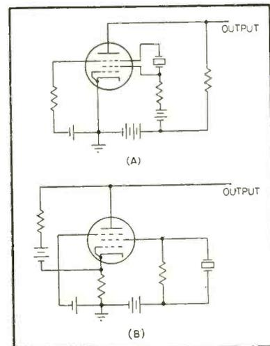
FIG. 1—Two crystal oscillators using only resistances as circuit components
