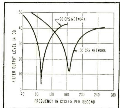
FIG. 2—Attenuation characteristics of the parallel-T filters
