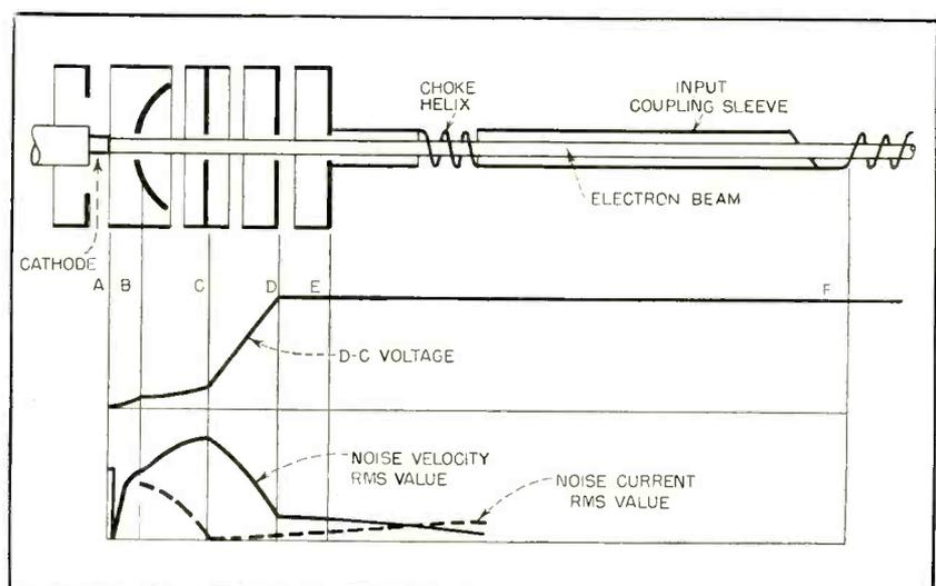
FIG. 4—Design principles employed in low-noise electron gun with three accelerating anodes
