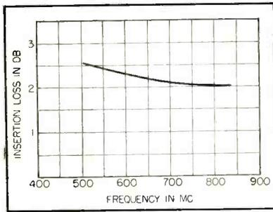
FIG. 2—Insertion loss for two cavities plotted against frequency
