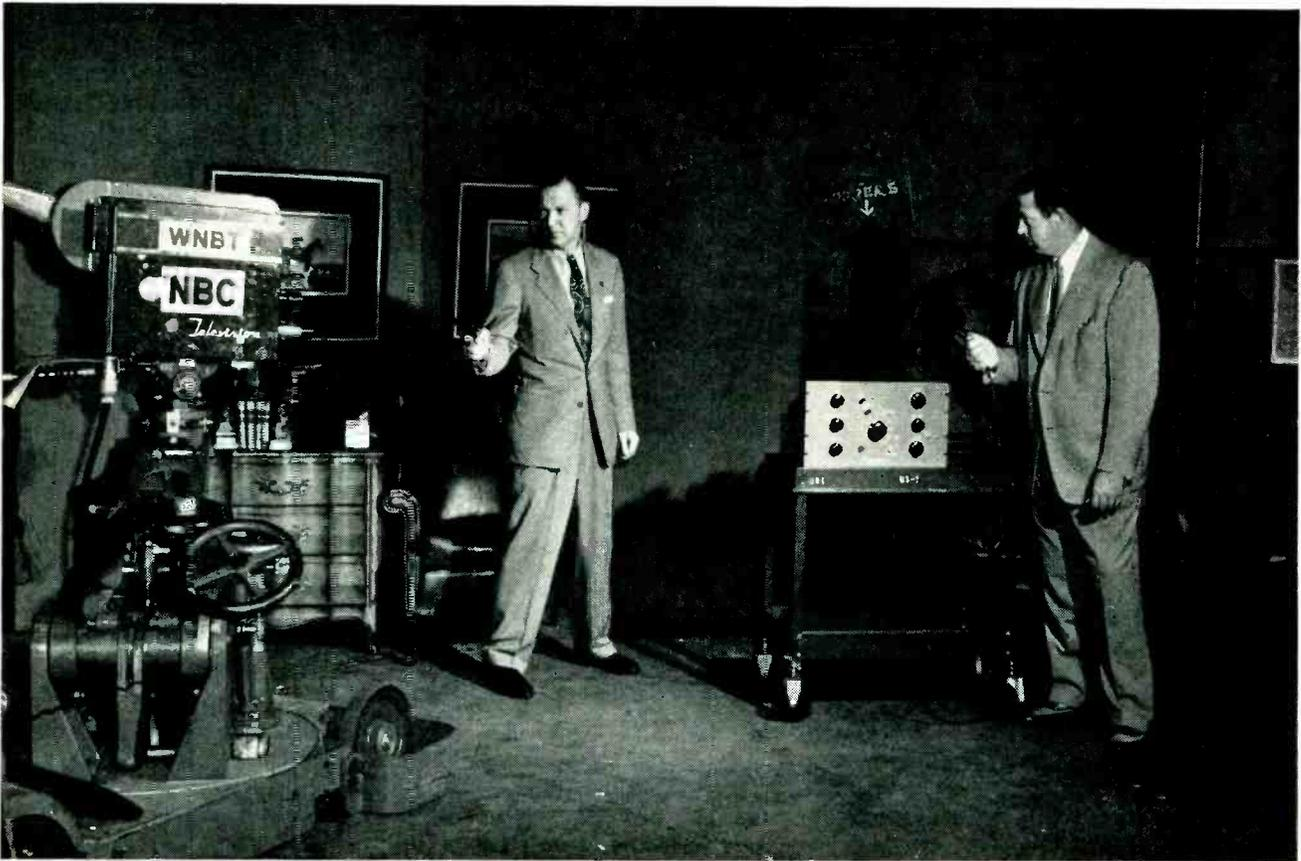
Method of using gunshot generator during television drama. Engineer at right holds single-shot pushbutton in hand and presses it when television detective Martin Kane pulls trigger of unloaded gun
