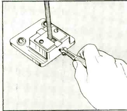
**2** Applicator withdrawn (new ring automatically feeds into place).
