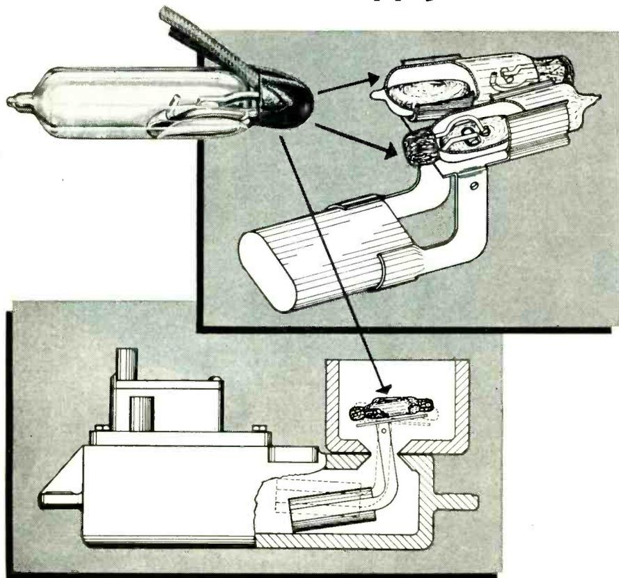
HONEYWELL mercury switches meet the demands for low operating force and have the additional advantage of contacts being sealed in a glass case, protected from effects of oil fumes.
