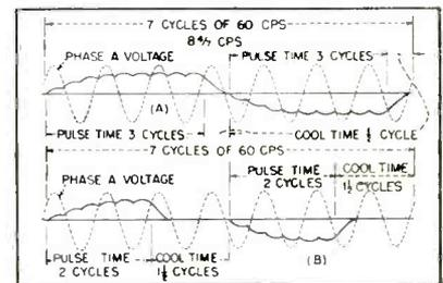
FIG. 3—Illustration of terms pulse time and interpulse time
