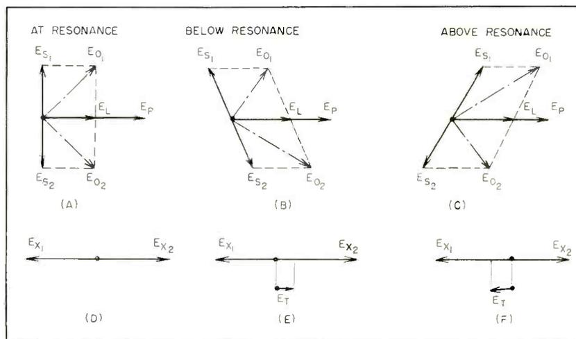
FIG. 2.—Vector voltages, resultant rectified voltages and output voltages for standard discriminator
