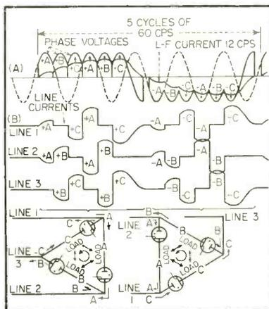
FIG. 1—Basic principle of converting three-phase power to single-phase low-frequency power by using power tubes
