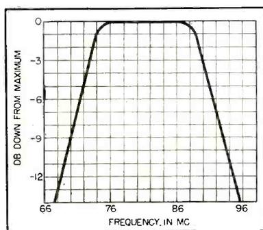
FIG. 5—Overall i-f response curve of converter
