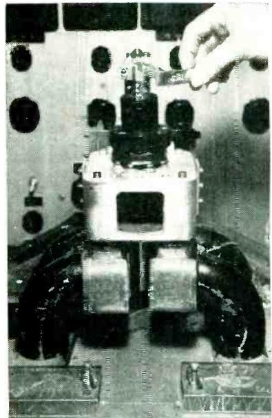
Method of locking subminiature tube in position, and construction details of exciter
