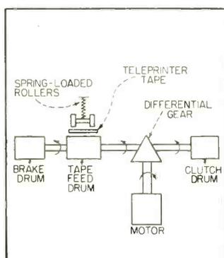
FIG. 1—Tape feed mechanism
