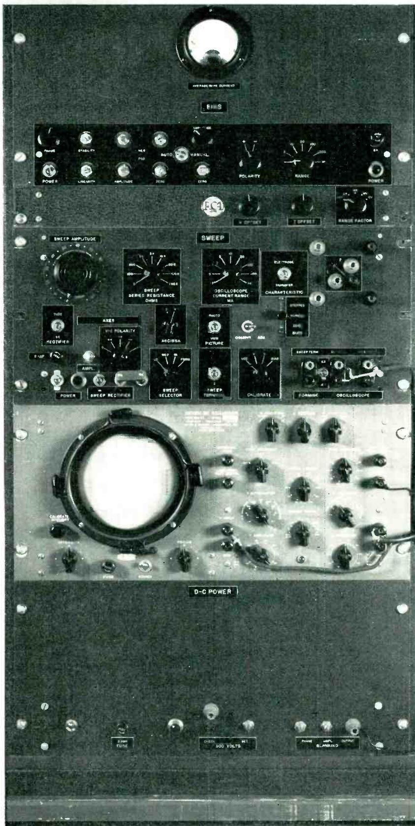
Curve tracer consists of four separate chassis. Transistor is connected to triple receptacle at right of sweep chassis; characteristics are displayed on scope face
