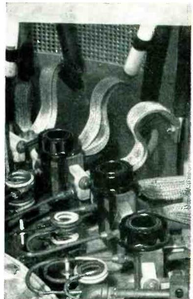
Electronic heating generators here speed production of pencil triodes, appearing here as tiny vertical white rods under the work coils
