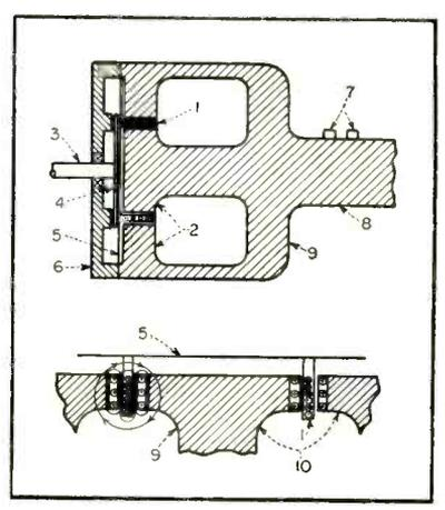
FIG. 1—Cross-sectional view of loud-speaker type clutch showing (1) actuating coil, (2) magnetic poles, (3) output shaft, (4) output disk, (5) flexible diaphragm, (6) backing disk, (7) slip rings for actuating current, (8) input shaft, (9) magnetic structure, (10) compensating coils. Lower diagram shows placement and action of compensating coils
