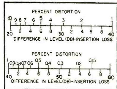
FIG. 2—Alignment chart for converting decibels to percent distortion
