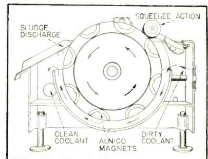
Cross-section of separator, showing how U-shaped Alnico magnets are mounted inside drum
