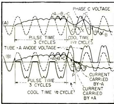
FIG. 4—Cause of commutation faults (A) and prevention of commutation faults by applying inversion operation (B)
