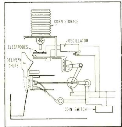
FIG. 8—Corn popper uses r-f to explode kernels in plastic bag. Alternative system pops corn, bags it later
