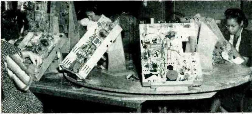
Turntable on pass-along assembly line for television receivers
