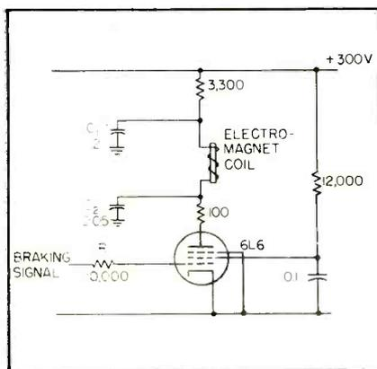
FIG. 4—Solenoid control circuit
