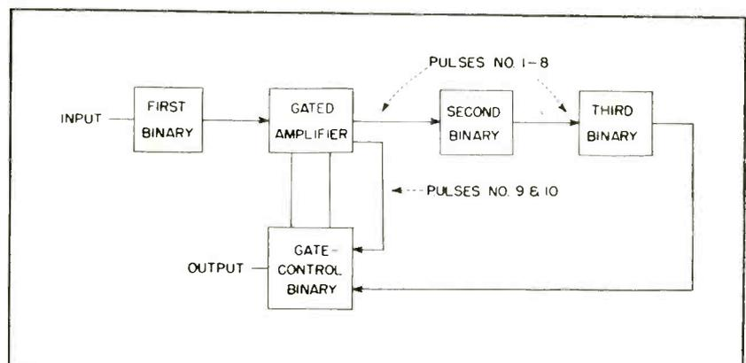
FIG. 1—Decade counter uses electronically-switched gate. Eighth input pulse trips gate; tenth pulse resets counter
