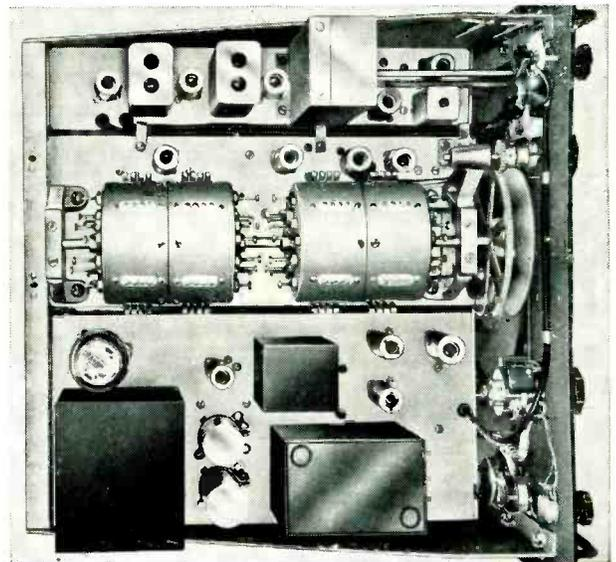
ing the coils. The complete assembly is suspended between two cast bronze brackets for rigidity.
