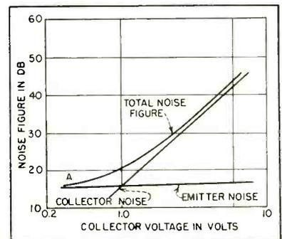
FIG. 8—Contribution to noise figure due to emitter and collector noise
