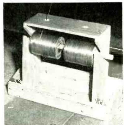
Simple holder for two spools of solder. Compartments at ends hold soldering iron tips
