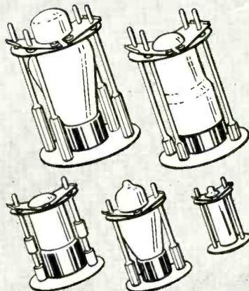
These retainers are used to secure Vacuum Tubes and to resist side motion of Vacuum Tubes used in radio equipment which is subject to shock and vibrations. These retainers meet the requirement of all JAN specifications. The insulated portion is made of a melamine base Fibre Glass Phenol which provides 300 volts insulation to ground and withstands a temperature of 350 F. The insulated plate can readily be fastened or released by hand.
