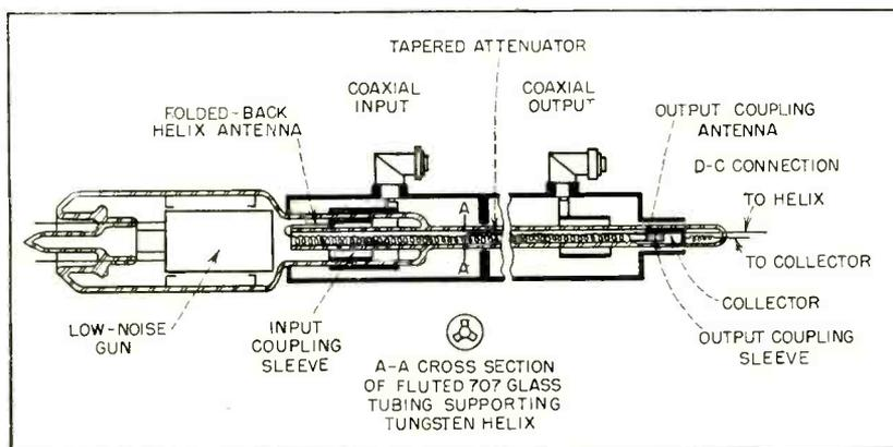
FIG. 3—Cross section of the tube shown in Fig. 2 with coaxial input and output matching transformers
