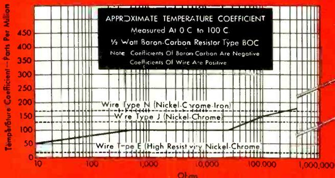
Type BOC conforms to all requirements of MIL-R-10509. Exposed to a temperature of 65°C. for one hour, the new BOC shows a resistance change of less than .2%. High temperature operation with reliability is now possible. Voltage coefficient is less than 20 parts per million per volt. Load life is outstanding; on a 500-hour test at ambient temperature of 40°C., resistance change will not exceed 2%.
