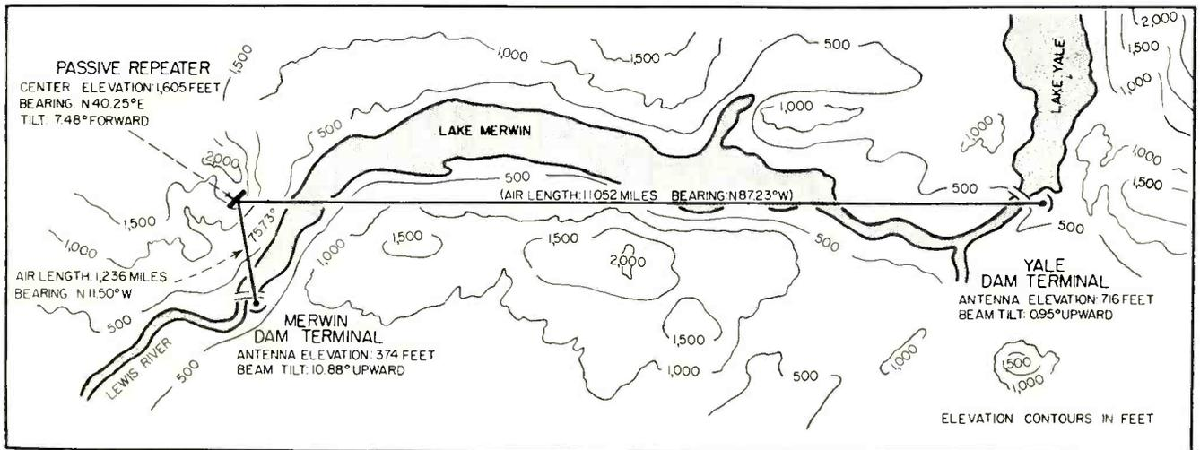
FIG. 2—Map of Lewis River, Washington, region shows how topography affects microwave control and communications between new Yale Dam and existing Merwin Dam downriver
