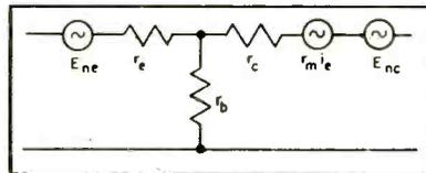
FIG. 2—Equivalent circuit of transistor including two noise-voltage generators
