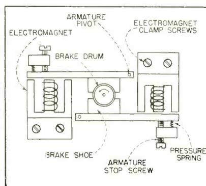
FIG. 2—Arrangement of brake
