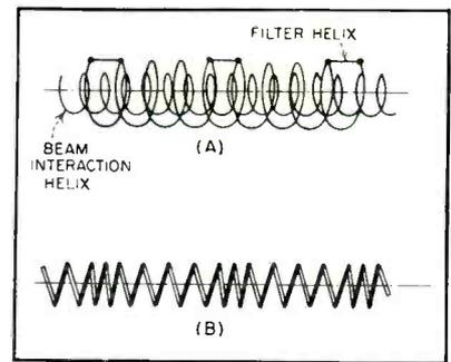
FIG. 9—External filter helix (A) can be changed to select operating frequency of tube containing inner helix or impedance discontinuities can be introduced by changes in helix pitch (B)
