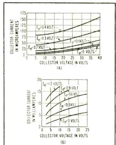
FIG. 7—Collector voltage versus collector current
