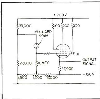
FIG. 5—Photoelectric reading stage
