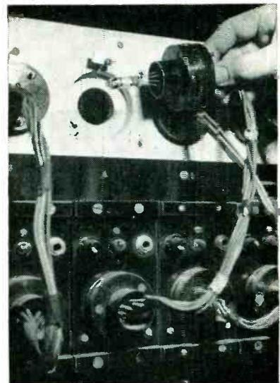
Method of supporting subminiature tube in life test oven. Swinging metal tab above hole in oven locks socket in position. Neon lamp on panel below indicates shorts, and jack permits monitoring of tube current at 500-hour intervals during the run.
