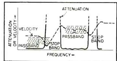
FIG. 10—Phase velocity versus frequency for a filter helix
