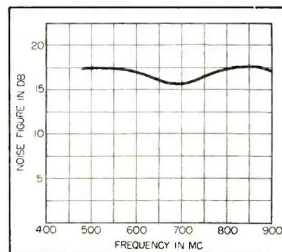
FIG. 7—Noise figure over the tuning range
