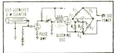
FIG. 10—Frequency meter measures discharge of Geiger tube
