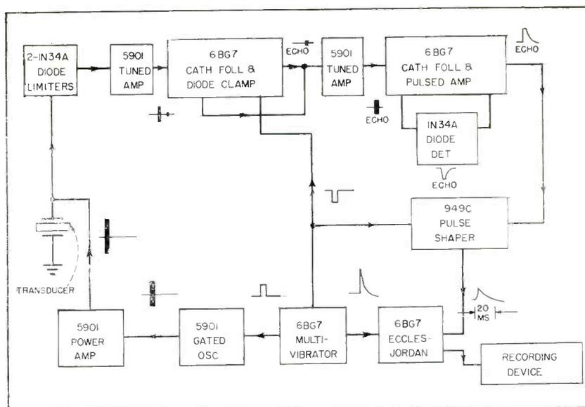
FIG. 2—Depth recorder employs ultrasonic transceiver. Variable-width pulse from Eccles-Jordan measures transit time of ultrasonic pulse reflected at air-water interface
