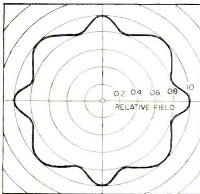
Calculated patterns for 90-degree skewed antenna
