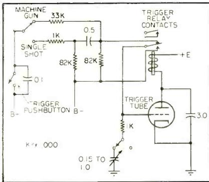
FIG. 3—Circuit used to obtain either single-shot effect or machine-gun sounds
