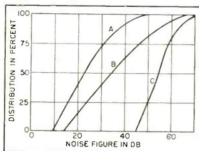
FIG. 4—Distribution of noise figure for 60 transistors of both types: A, junction transistors with  $V_c = 1$  v and  $I_c = 0.5$  ma; B, junction transistors at  $V_c = 5$  v and  $I_c = 1$  ma and C, point-contact transistors at  $V_c = 10$  v and  $I_c = 0.5$  ma
