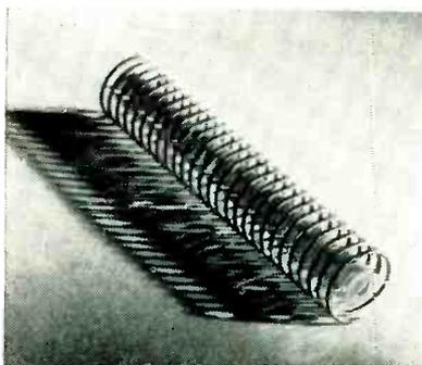
FIG. 8—Internal structure gives filter characteristic
