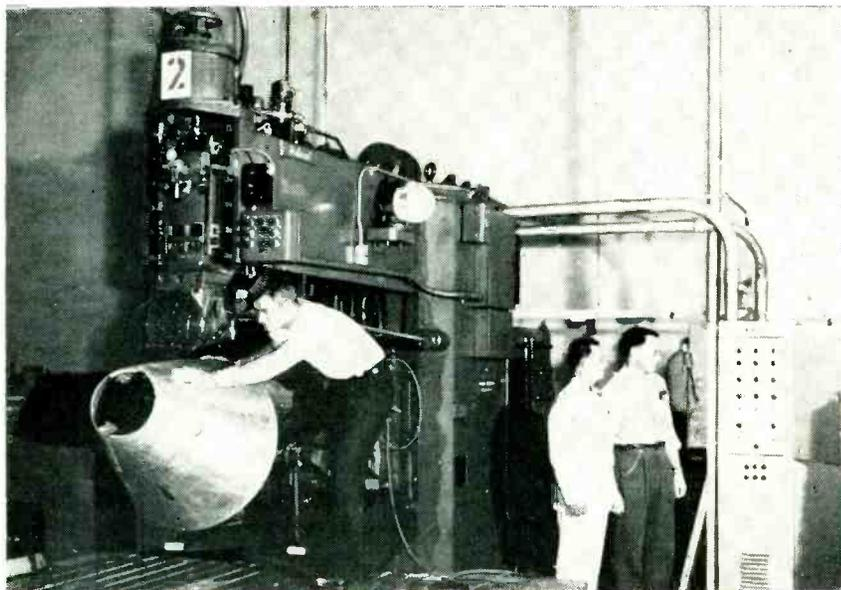
Three-phase resistance welding control (right) used with a spot-welding machine at a West Coast aeronautical plant
