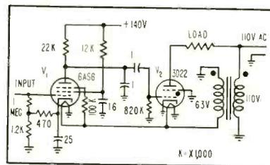
FIG. 1—Diagram of thyatron control circuit using out-of-phase suppressor grid voltage as trigger control
