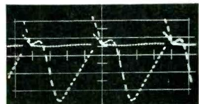
(A) The effects of negative grid swing (lower wave) on conduction period. (upper wave). As negative swing is increased conduction period is shortened
