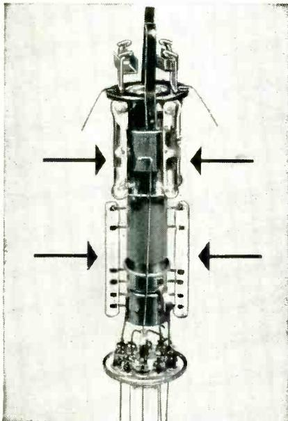
**Improved Gun Employs Glass Beads.** Westinghouse makes the new metal cone electrostatic focus tube with glass-beaded assembly. This assures accurate element spacing within close tolerances to improve spot size and picture uniformity.
