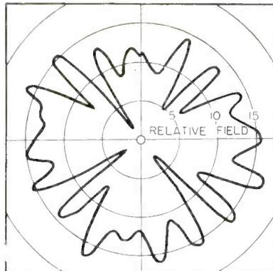
Measured patterns for antenna without skew
