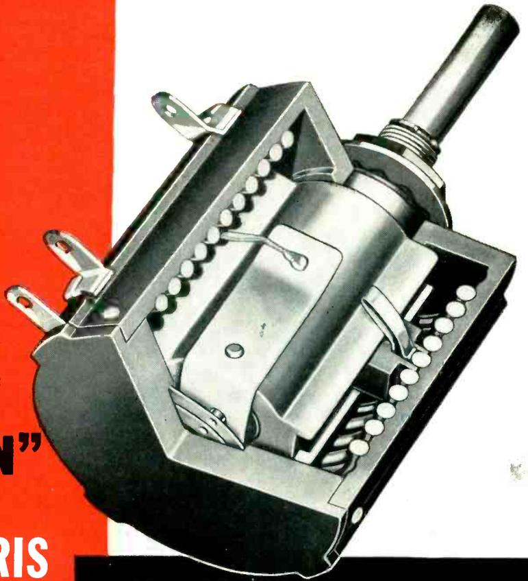
Cutaway view of Model A 10-turn Helipot precision helical potentiometer. Resistance element 45" long is contained in case  $2" \times 1\frac{13}{16}"$  diameter. On element are wound 3000 to 9800 turns of resistance wire, depending on total resistance value required. Adjustment accuracy is 12 to 14 times that of conventional single-turn potentiometer of equal diameter.
