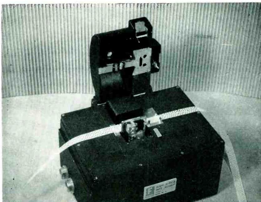
Tape reader, with lamp housing lifted to show feed mechanism
