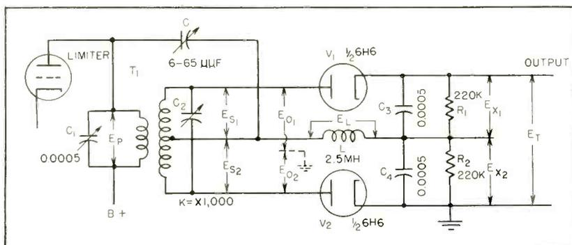
FIG. 1—Conventional discriminator is modified for narrow-band f-m by changing values of  $L$  and  $C$  to resonate above  $T_1$  primary
