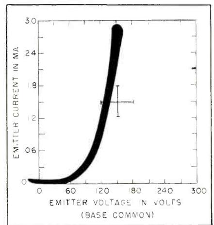
FIG. 8—Family of emitter characteristics
