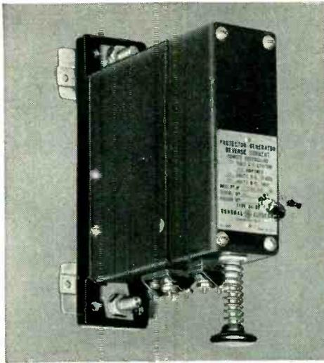
**CIRCUIT BREAKERS**—Here, a Carboloy magnet assembly simplifies trip element. It eliminates a coil and polarizing connection . . . makes possible reverse-current tripping independent of system voltage. Breaker weighs less, costs less to build, eliminates nuisance trips in circuits.
