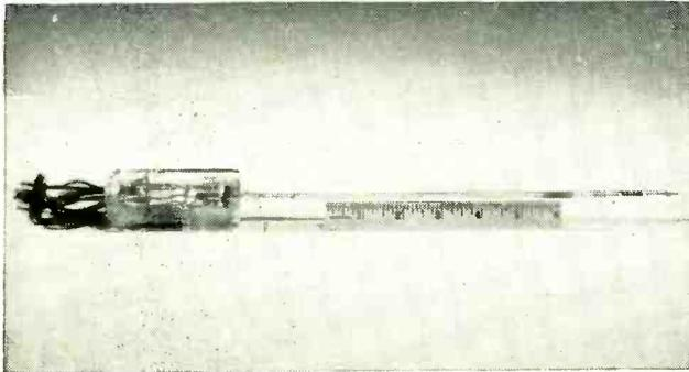
FIG. 1—Conventional traveling-wave tube with low-noise gun operates at 500 volts beam potential
