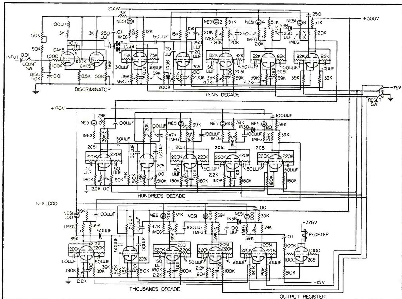
FIG. 5—Nuclear scaler uses input discriminator and three gated decades to count particles in radioactive decay. Four-light interpolation is used
