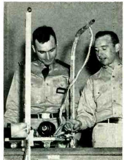
FIG. 1—Target simulator used in radar training. Echo box at lower left reflects radar waves to give same scope pattern as a plane in flight
