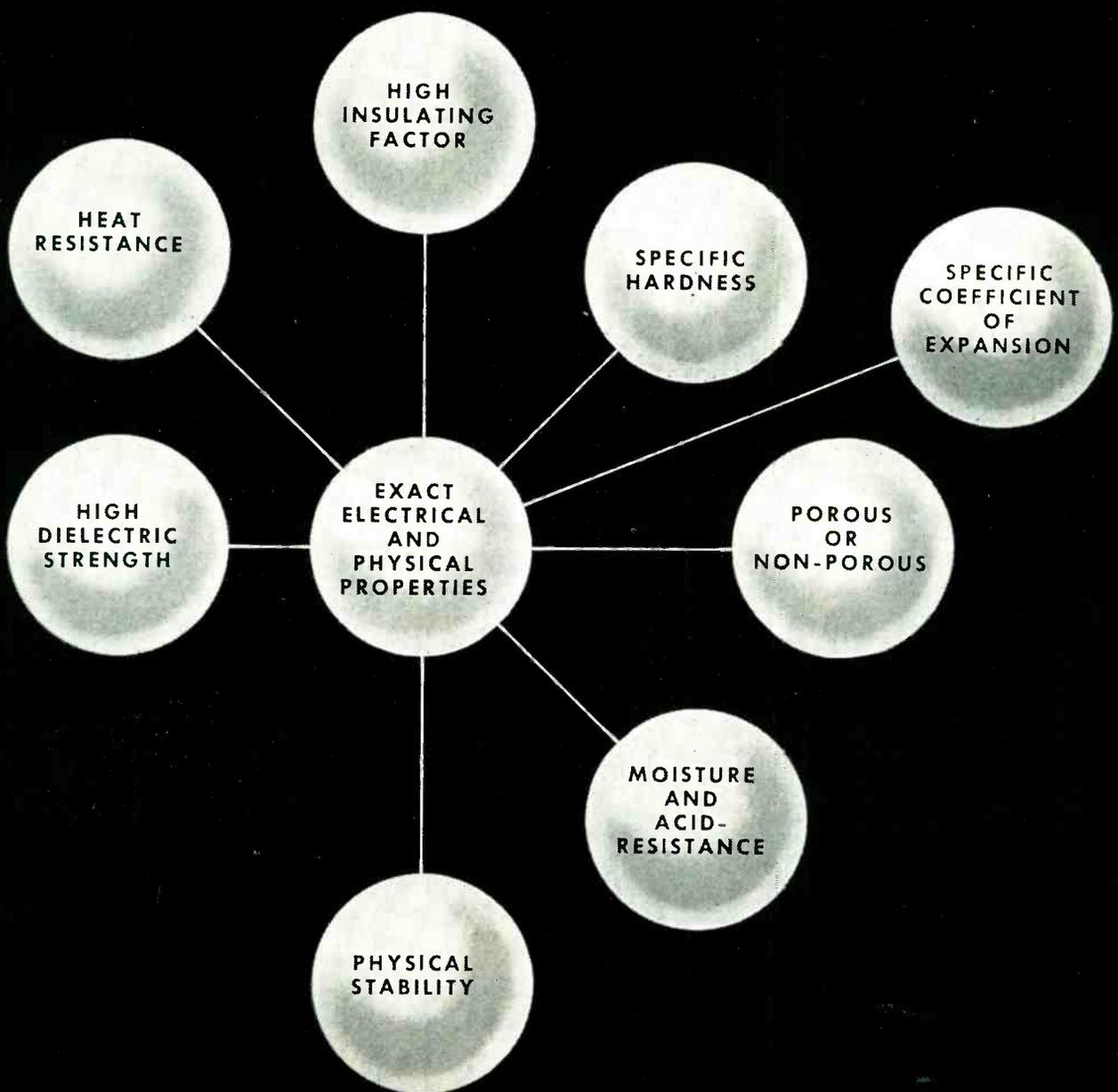
**T**HERE'S a Centralab Ceramic material to match your individual requirements — electrically . . . physically . . . structurally. These materials are unique. We can extrude, mold or press them. What's more, Centralab Ceramics can be worked the same as metal—drilled, turned, ground or tapped. In addition, they can be metalized. Every Centralab Ceramic has some of the properties shown above, and they meet all
