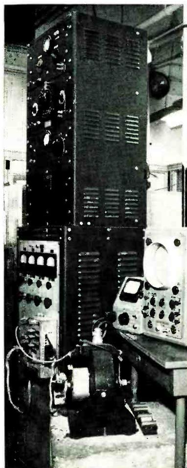
Laboratory-type vibration test setup used for sampling inspection of tubes. Exciter is mounted on concrete block to minimize extraneous vibrations
