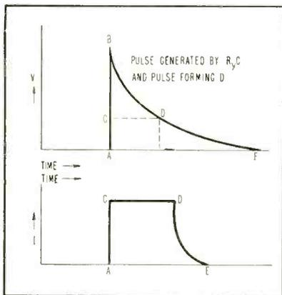
FIG. 2—Pulse forms required for dental testing
