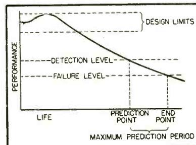
FIG. 1—Chart showing deterioration in performance during life of component. This type of curve is applicable to many types of components including tubes, resistors, capacitors or complete subassemblies
