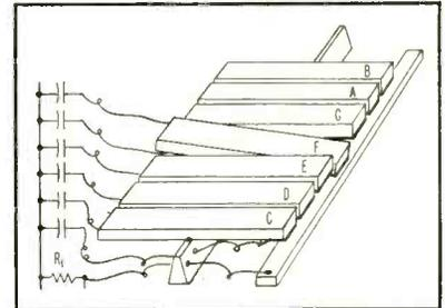
FIG. 2—Wooden keys of toy piano are modified as shown to serve as spst switches for playing notes of transistor organ
