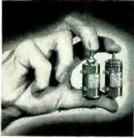
Series AJ Helipot models are only  $\frac{3}{4}$ " in diameter and  $1\frac{3}{8}$ " long; weight 1.0 oz. Ten-turn 18" slide wire gives adjustment accuracy of 1/3000 in a 100-ohm unit—1/6500 in a 50,000-ohm unit.
