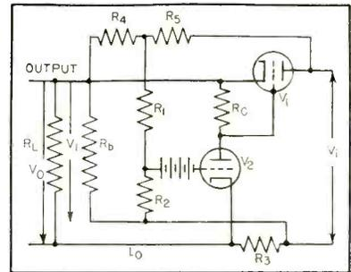
Circuit of zero or negative impedance power supply regulator
