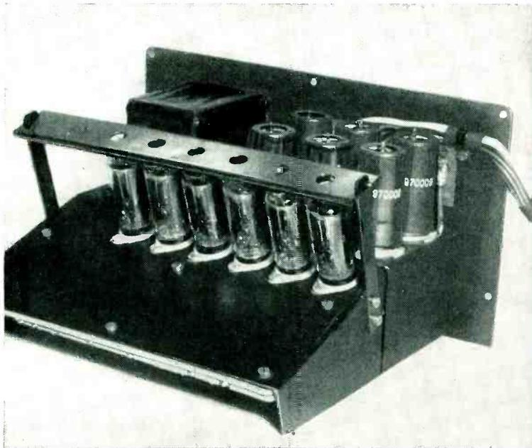
Six phototubes of system are in foreground, with cathode follower stages and power transformer behind. Optical system is in main housing, not shown
