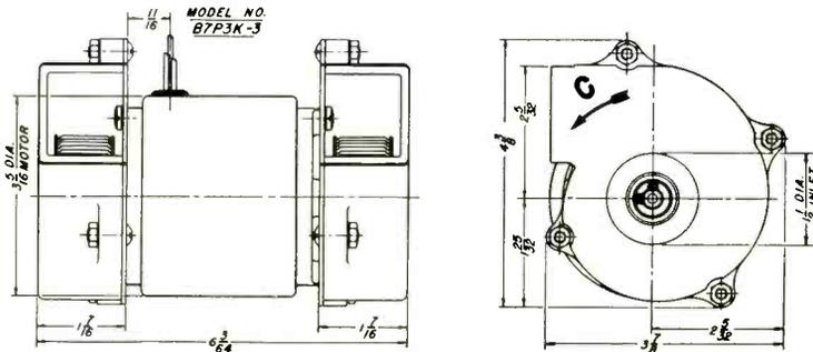
Maximum cooling for airborne radar and hot-running electronic equipment is assured with this compact double-ended centrifugal blower. It meets government specifications for use at altitudes up to 50,000 feet. Another illustration of EAD's design ability!
