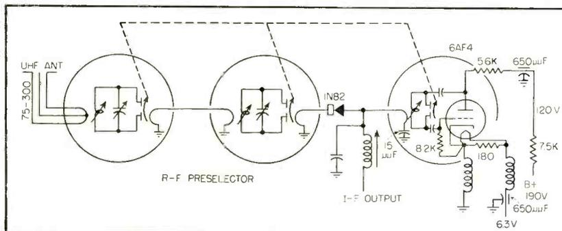
FIG. 1—Three cavities are employed, two for preselection and one for the local oscillator
