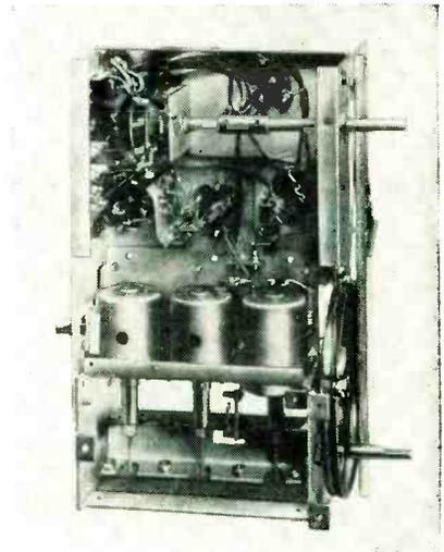
Ganged plungers move in and out of the cavities for tuning the complete uhf range
