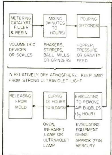
FIG. 1—General casting process for circuit and component embedment
