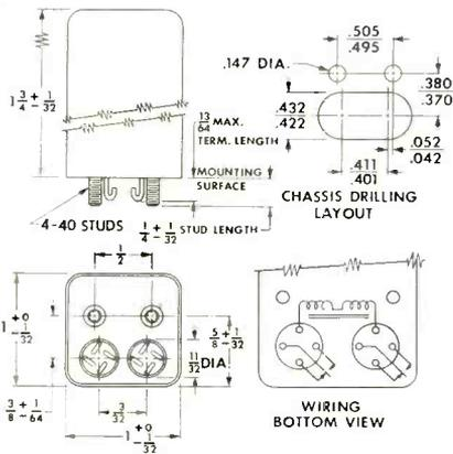
Contact arrangements up to and including DP DT 3 Amp at 28 volts D.C., or 100 Milliamperes at 150 volts D.C. resistive load.
