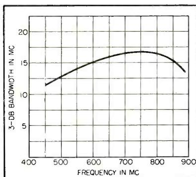
FIG. 6—Overall 3-db bandwidth for converter
