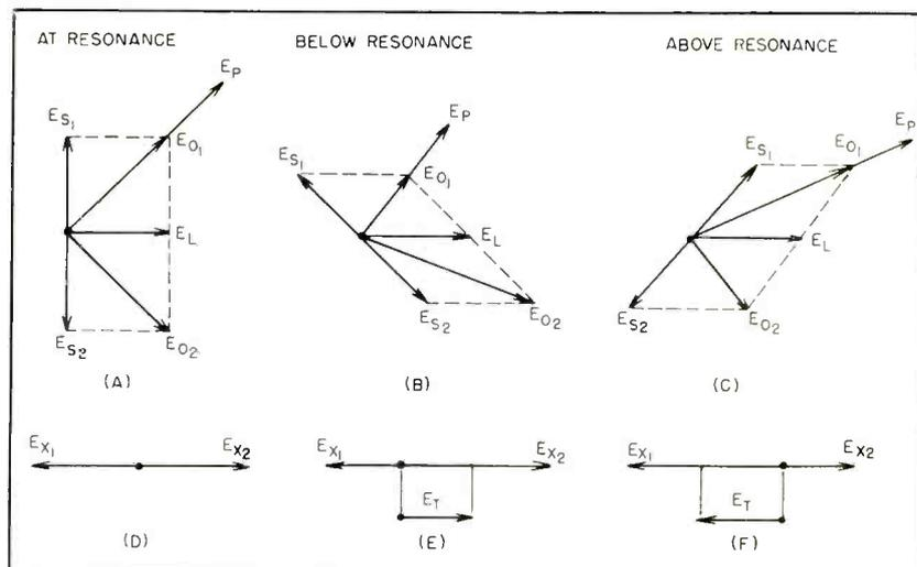
FIG. 3.—Voltages for modified Foster-Seeley circuit show increased output for slight frequency deviation
